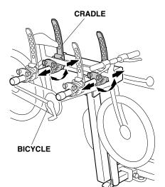
2. Install the two anti-sway cage assemblies to the bicycle arms as shown.
