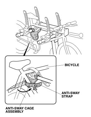
5. Using the strap provided, secure the bicycle wheels. Secure the strap buckle as shown.
