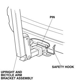
2. Gently lower the upright and bicycle arm bracket assembly to the stop position.
